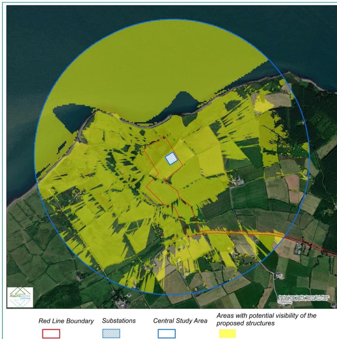
Figure 14.6: Digital Surface Model (DSM) based ZTV map accounting for screening by surface elements such as hedgerows and trees lines.
